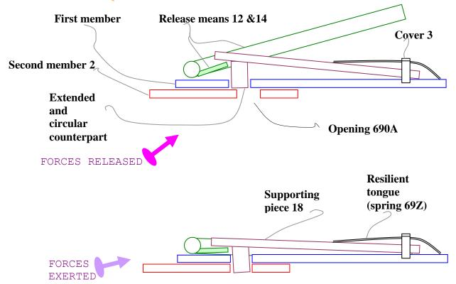
How it works: The pin supporting piece 20, "floats" on the outer square tube (first member 1). A cover 3, about 6" long, is a U shaped piece; it goes over the resilient tongue, which is a leaf spring. It also goes over the supporting piece, and makes it look good, and limits pin movement. Pry rod 22 & plate 3 pry the pin out.
