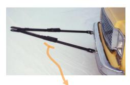
This is a telescoping tow bar, so its easy to hook up. It is rated at 5,000 lbs. and has a pressure release latch developing about 14:1 leverage, so its easy to unhook.
