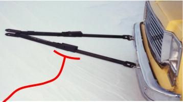
Left drawing; the operator backs up before unhooking. This compresses the rollers in the tow bar latch.
