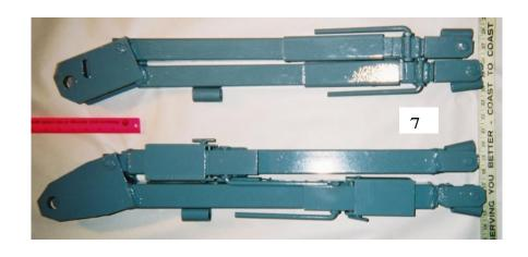
In picture 7 the top tow bar is the standard tow bar.
