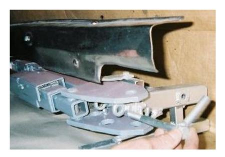
When the tow bar is folded in, above right, a <u>longer</u> pin with a welded extension member is inserted in the eyebolts.
