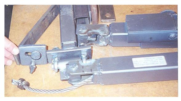
The cable goes through the center of the telescopin g tow bar arms.
