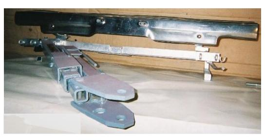
In the towing position, the standard is 41  $\frac{3}{4}$ " long, the Brute is 44  $\frac{1}{2}$ " long.
